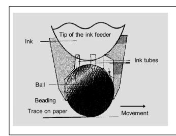
To ensure the ink transfer by capillary forces whilst writing, the suitable distance between ink feeder and ball is about 0.02 to 0.05 mm.
