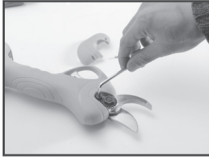
2. Remove the screws on the nut pin (this step is critical)
